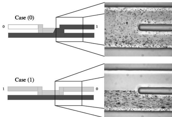
FIG. 1. Illustration and experimental realization of a microfluidic-based NOT gate where the 100  $\mu\text{m}$  outlet channels fabricated in PDMS are shown.
