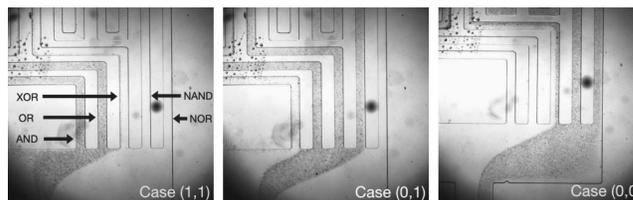
FIG. 3. Experimental realization of the illustration of Fig. 2 where only the outlet channels are shown. Note some spillover into the XOR gate.
