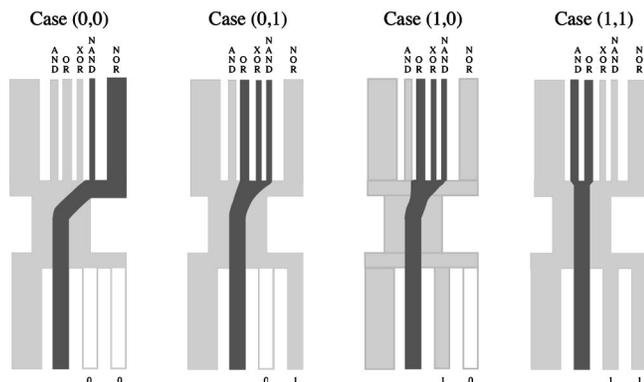
FIG. 2. Multigate design where the output channel width reflects its relative flow resistance (see Table I) and not the actual width. Note that with all five logic gates actuated simultaneously, combination of the XOR and AND gates constitutes a half-adder.
