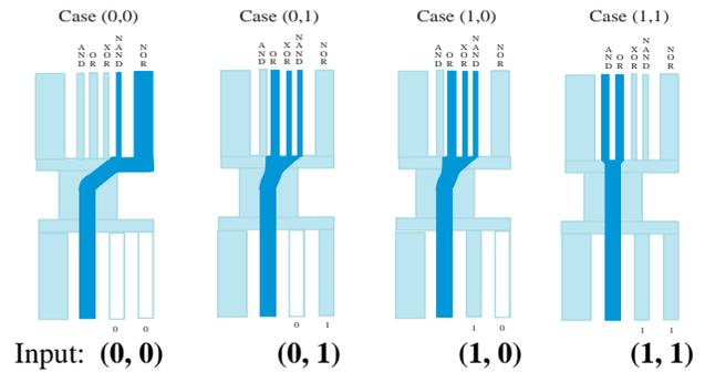
Figure 3. Experimental realization of the illustration of Figure 2. Only the output channels of Fig. 2 are shown. The diameter of each channel is approximately 100 microns. Channel structures could be scaled down to 50 nm using related lithographic techniques.
